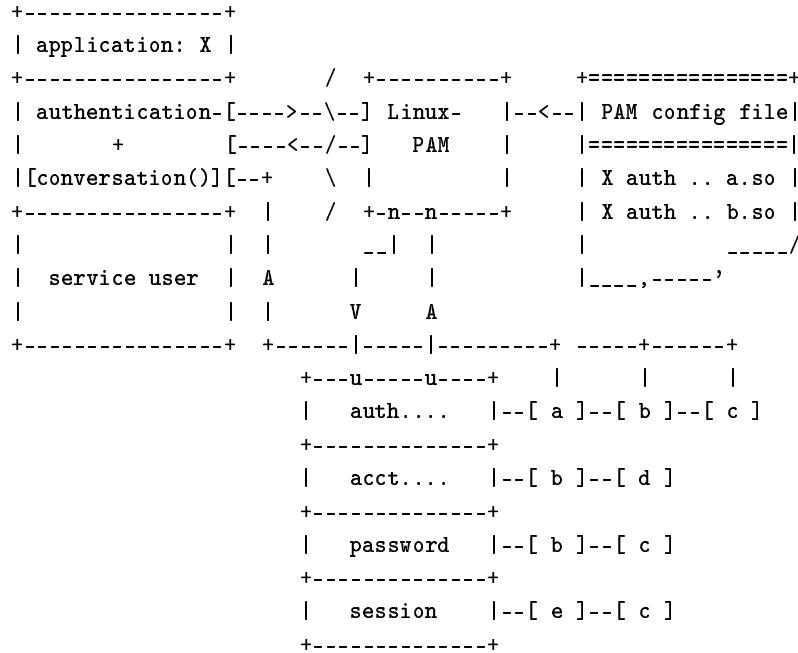
By way of explanation, the left of the figure represents the application; application X. Such an application interfaces with the **Linux-PAM** library and knows none of the specifics of its configured authentication method. The **Linux-PAM** library (in the center) consults the contents of the PAM configuration file and loads the modules that are appropriate for application-X. These modules fall into one of four management
