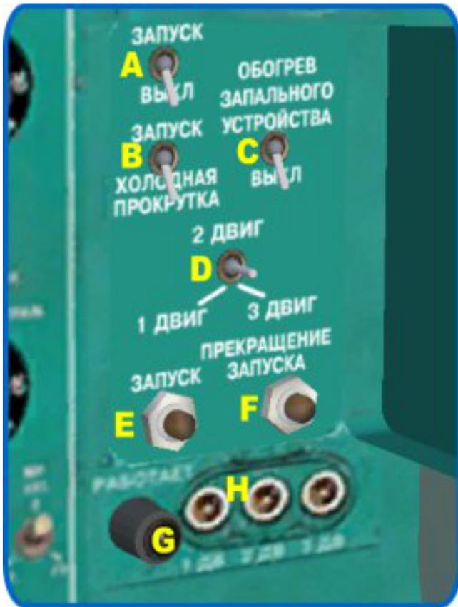
Fig. 12. Engine start panel
