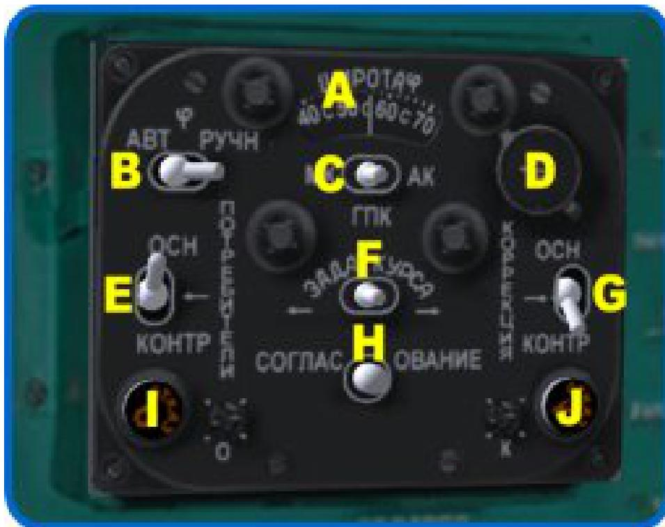
Fig. 5. PU-11 TKS compass system.
