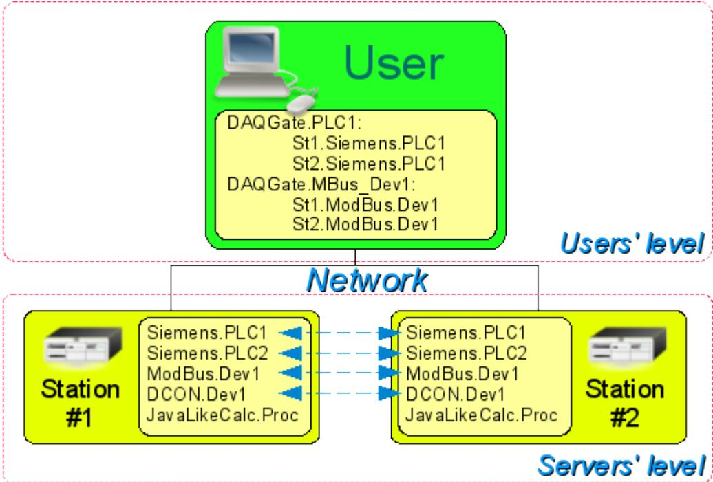
Fig.1. Horizontal and vertical redundancy.
