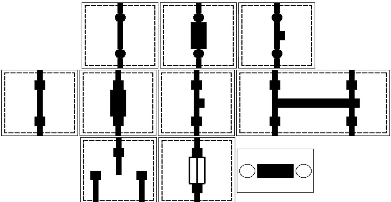
Fig.1. Elements from left to right from top to bottom: "Switch plank(circle)", "Fuse-switch(circle)", "Automatic switch plank(circle)", "Switch plank", "Fuse-switch", "Automatic switch plank", "Automatic dual band switch", "Switch with the neutral central position", "Fuse-switch 2", "Switch".
