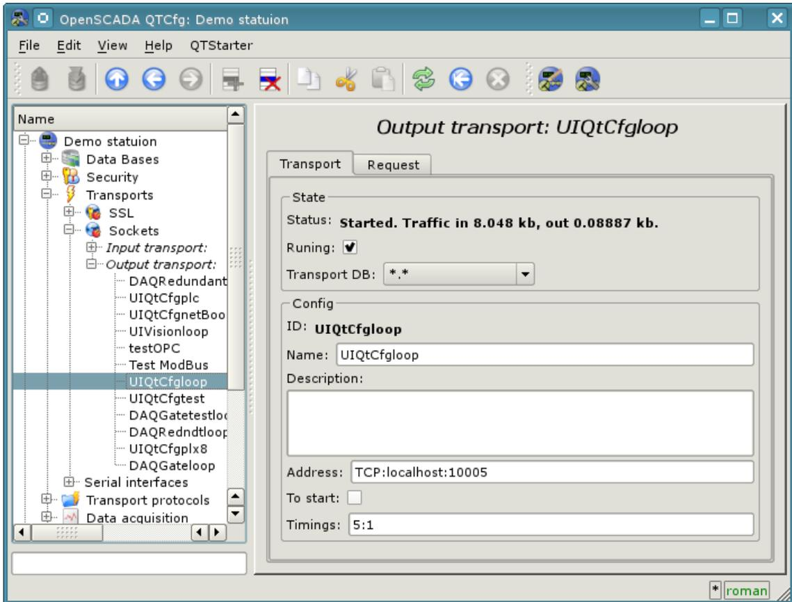
Fig.2. Main tab of the configuration page of the outgoing socket.
