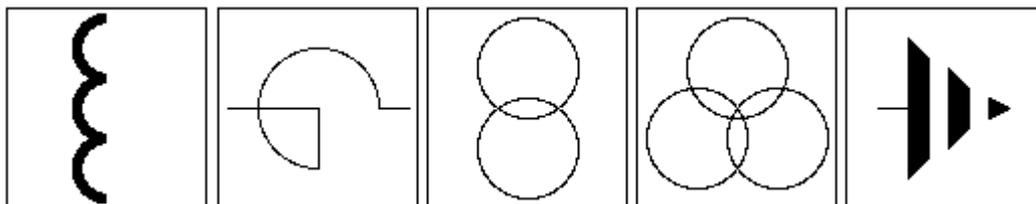
*Fig.3. Static elements from left to right: "Coil", "Reactor", "Transformer", "Transformer with two secondary windings", "Ground".*
