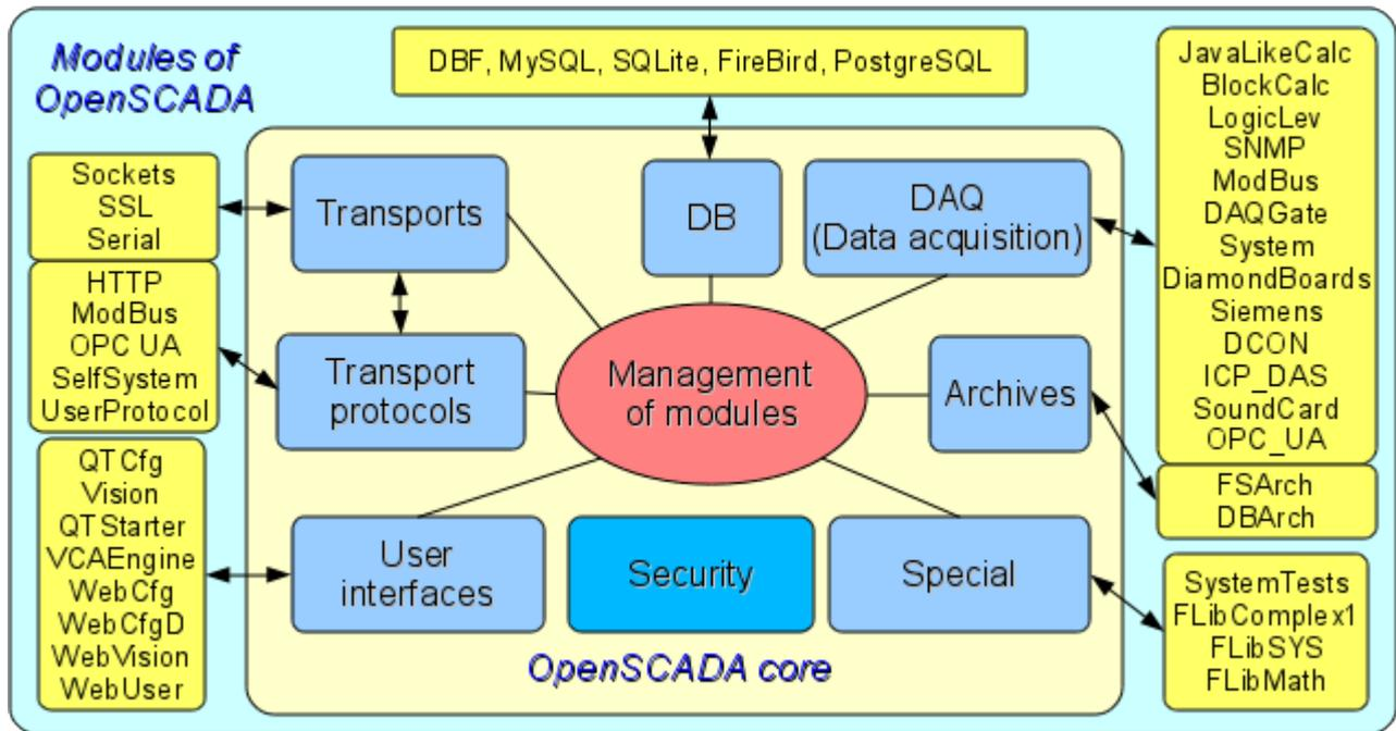
Fig. 1. The block scheme of OpenSCADA system
