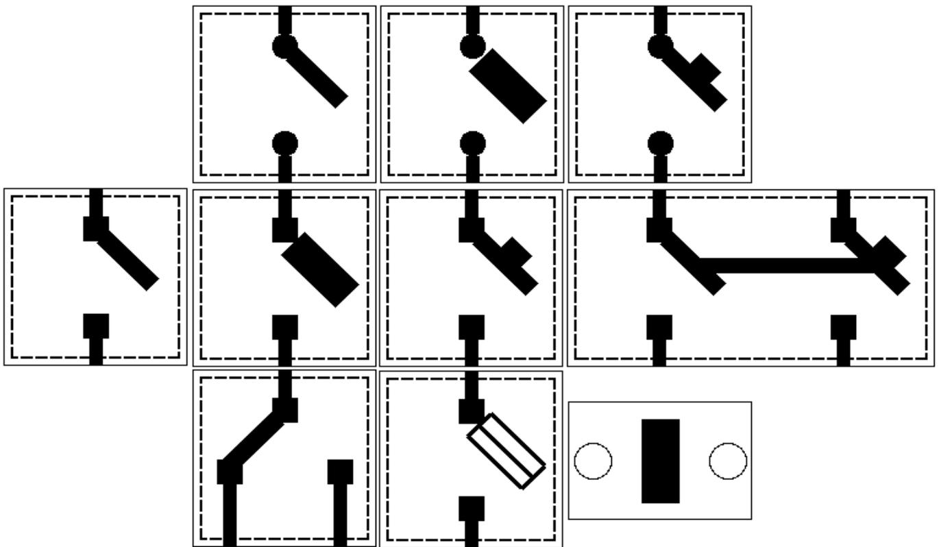
Fig.2. Elements from left to right from top to bottom: "Switch plank(circle)", "Fuse-switch(circle)", "Automatic switch plank(circle)", "Switch plank", "Fuse-switch", "Automatic switch plank", "Automatic dual band switch", "Switch with the neutral central position", "Fuse-switch 2", "Switch".
