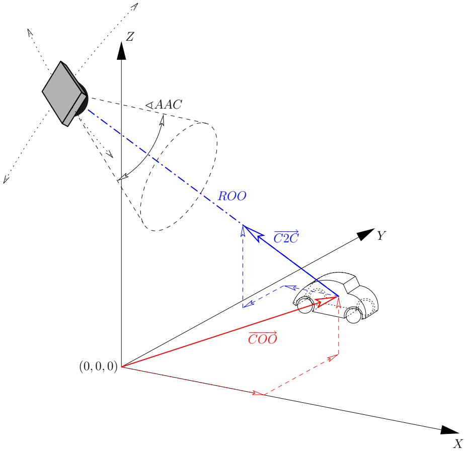
Figure 1: Camera and 3D object in the World System  $XYZ$ ; centre of orbit position vector  $\vec{COO}$ , centre of orbit to camera direction vector  $\vec{C2C}$ , radius of orbit  $ROO$ , aperture angle of camera  $\triangle AAC$ .
