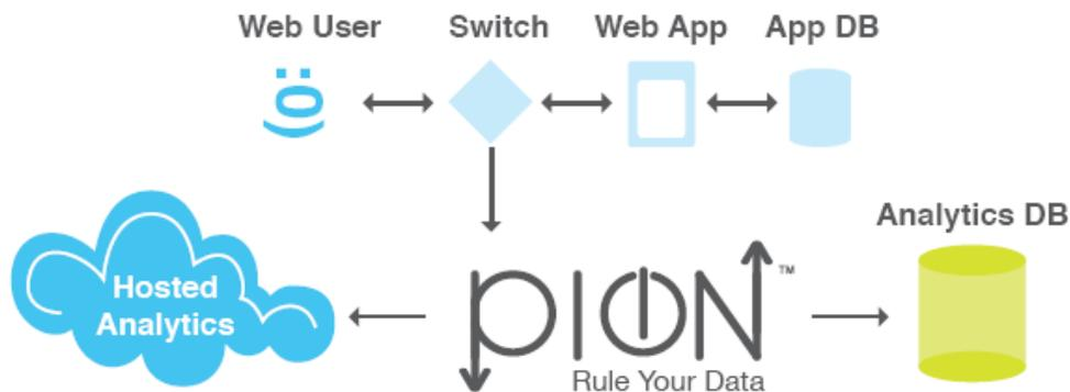
Note: The diagram is collapsed for Pion installed directly on the web server. Pion + Web App + App DB would all be in one box with arrows going to the switch, the Hosted Analytics Cloud and the Analytics DB bin.
