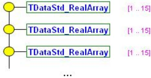
2. Allocation of data of each measurement point as arrays of double values
