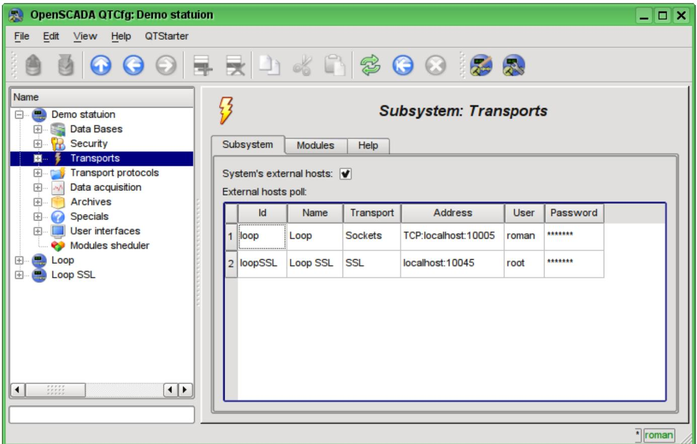
Fig. 13. The "Subsystem" tab of the "Transports" subsystem.
