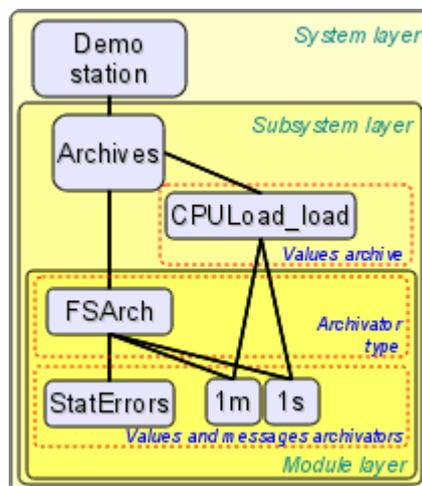
Fig. 5. The hierarchical structure of subsystem "Archives".
