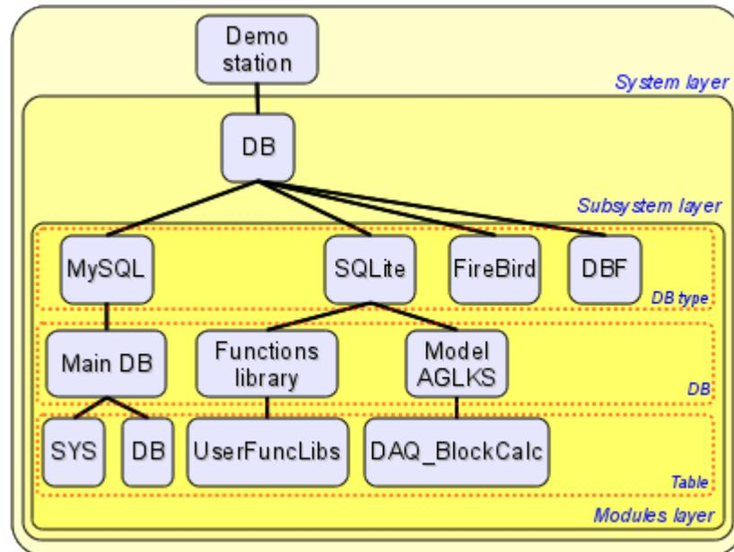
Fig. 3. Hierarchical structure of the database subsystem.
