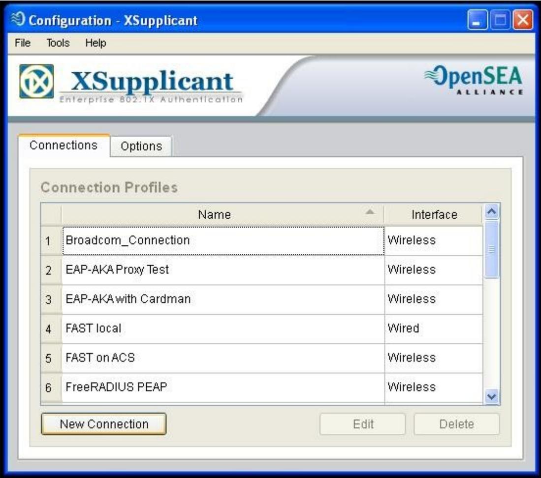
Click on the “New Connection” button to create a new AKA connection. This will bring up the first window in the configuration wizard.
