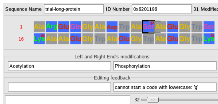
Figure 8.7: Bad code character in GNU polyxedit sequence editor. This figure shows the feedback that the user is provided by the code editing engine, when a bad character code is keyed-in.
