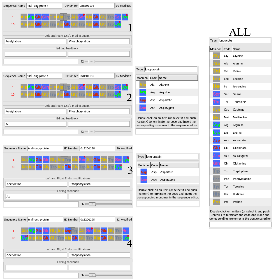
Figure 8.3: Multi-character code sequence editing in polyxedit . This figure shows the process by which it is made possible to edit polymer sequences with a code set that allows more than one character per code.
