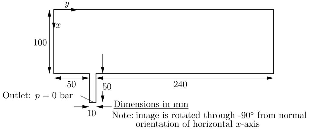
Figure 3.9: Geometry of a tank with outflow pipe
