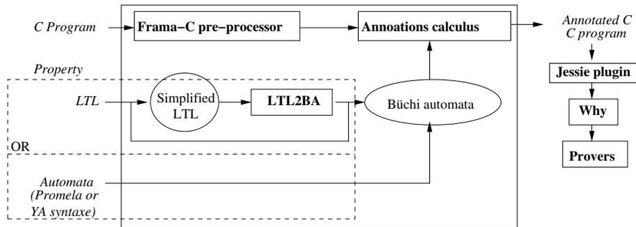
Figure 5.2: Plug-in Structure
