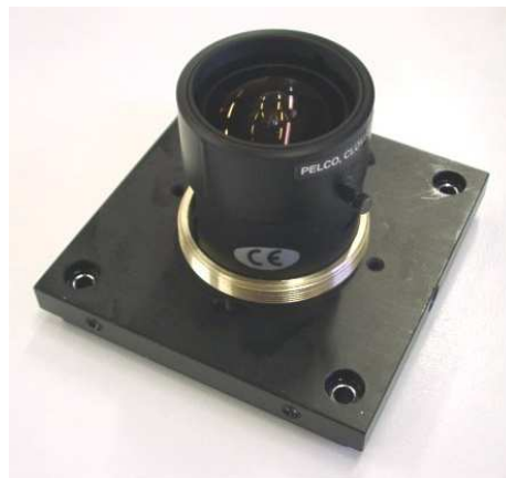
Figure 13 - Adapter between camera and optics
