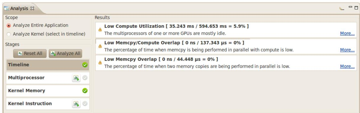
Analysis can be performed across the entire application, or for a single kernel instance. The type of analysis to perform is selected in the scope area of the Analysis view. When analyzing a single kernel instance, the kernel must be selected in the timeline.
