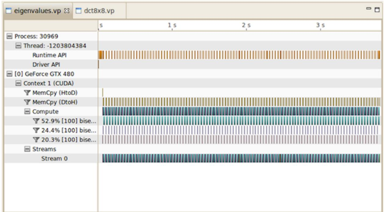
Along the top of the view is a horizontal ruler that shows elapsed time from the start of application profiling. Along the left of the view is a vertical ruler that describes what is being shown for each horizontal row of the timeline, and that contains various controls for the timeline. These controls are described in [Timeline Controls](#)
